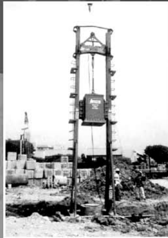
Patented Hydraulic Release PDA Test Hammer up to 15 ton Ram Weight
