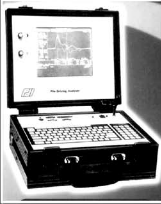
Dynamic Pile Testing-PDA System
